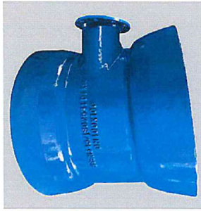
Double Socket Tees with Flanged Branch (Level Invert Outlet) PN25
