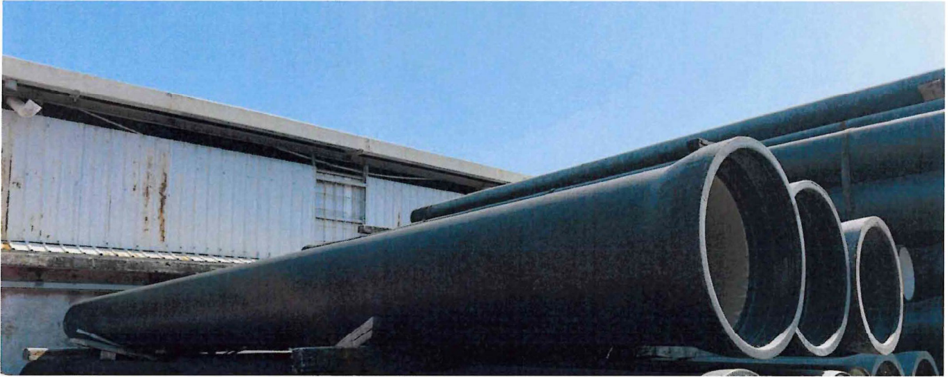
Ductile iron pipes with push in flexible joints (Class C and K)
