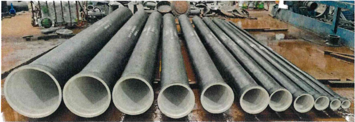
K9 Ductile iron socket and spigot pipes
